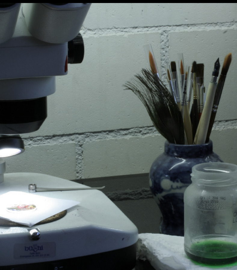
Microscope with a Magnification of 20 to 40 x, J-Variou brushes (synthetic brushes are considered as best), Aqua Regia oil. Kings Water (aqua regia) is a mixture of 3 parts Hydrochloric acid and 1 part concentrated nitric acid. With aqua regia also precious metal preparations for porcelain and glass painting are produced.
