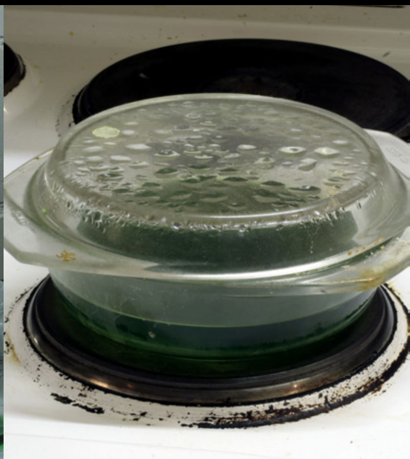
In a first step, the sapphire crystal must be cleaned, first boiled for one hour in Hydrochloric acid. In a second step the crystal is cleaned under clean water and then kept in the oven at 250°C over night.
