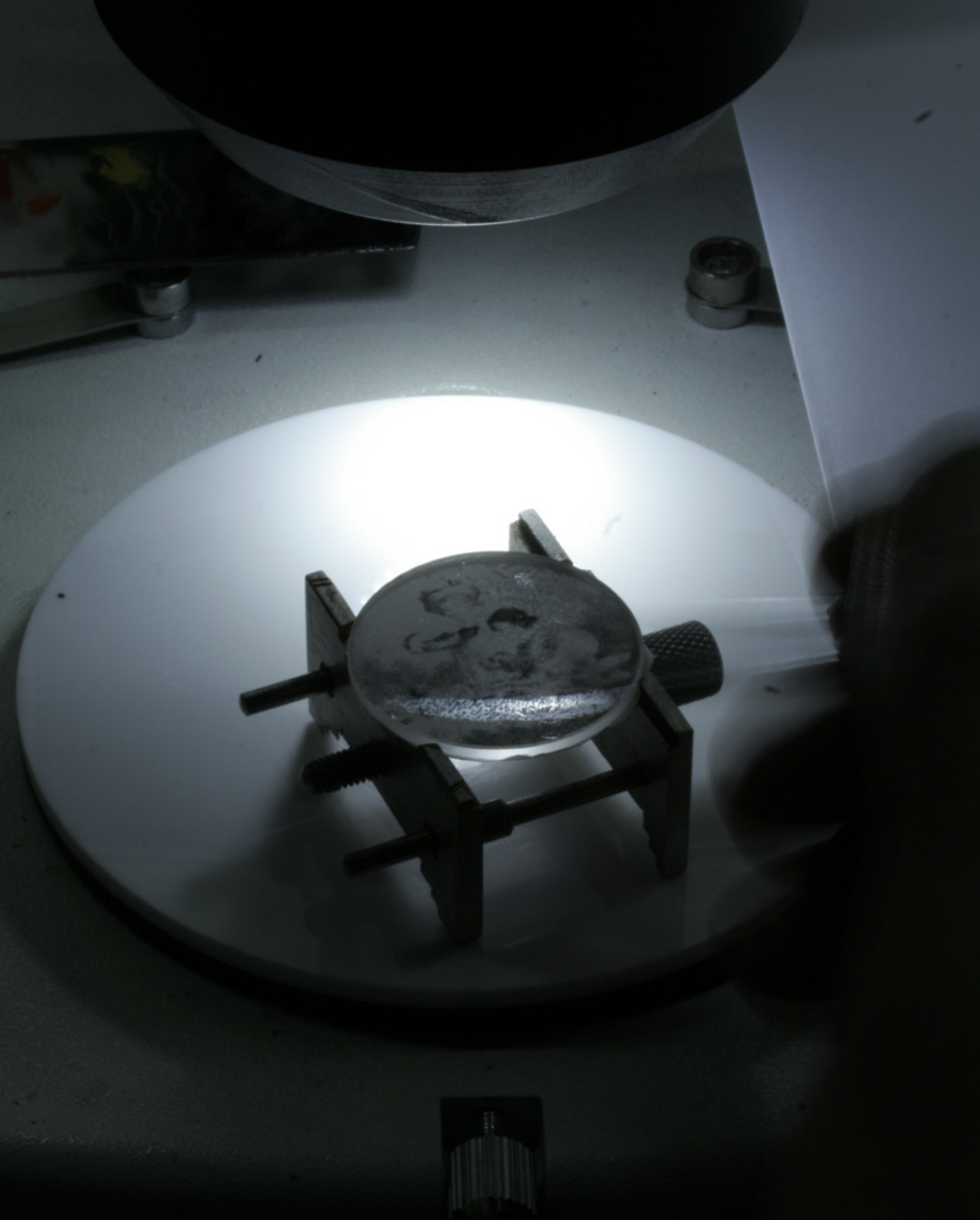
With a bush, a thin layer of oil is applied on the whole surface of the sapphire
