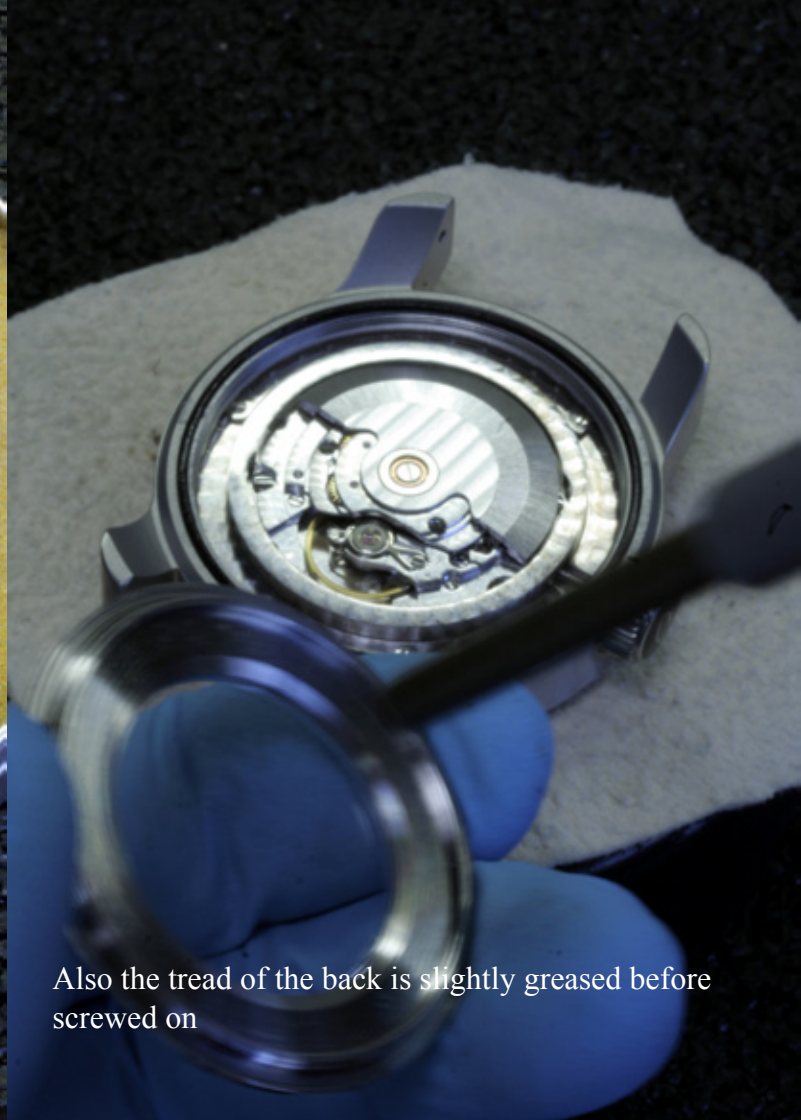
The O-ring is placed after being rubbed with Silicone grease
