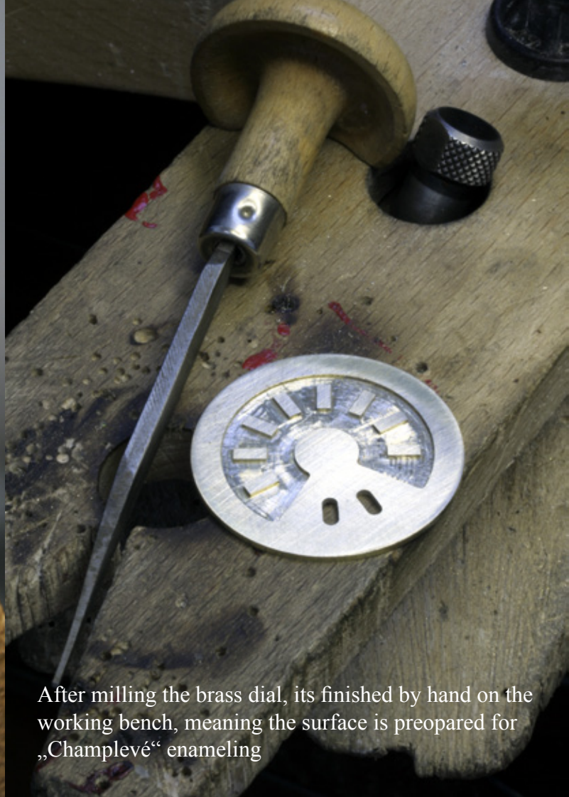
The dial is milled on the Pantograph milling machine
