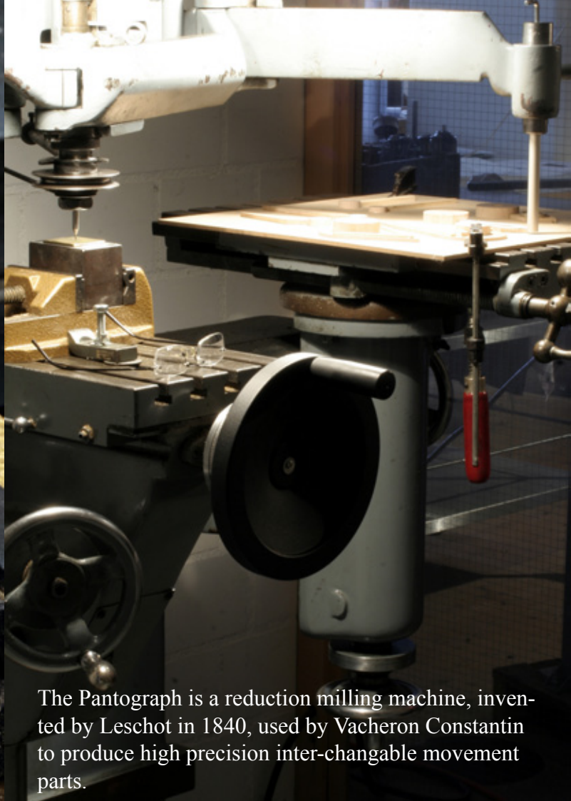
The hands are made in the same way as the dial on the Pantograph milling machine
