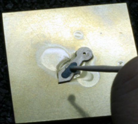
With a stick or tooth pick, some of the moisty enamel is set into the center hole
