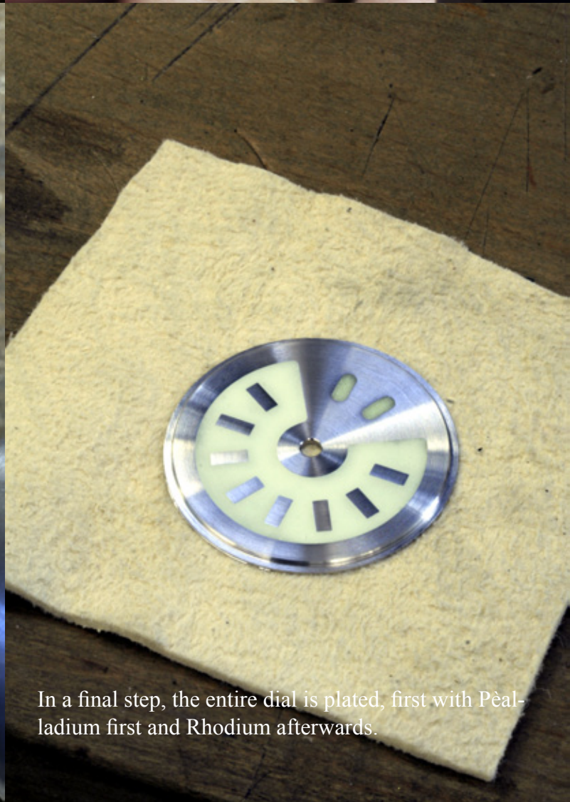
The contours are cut to fit the case and the center hole is drilled
