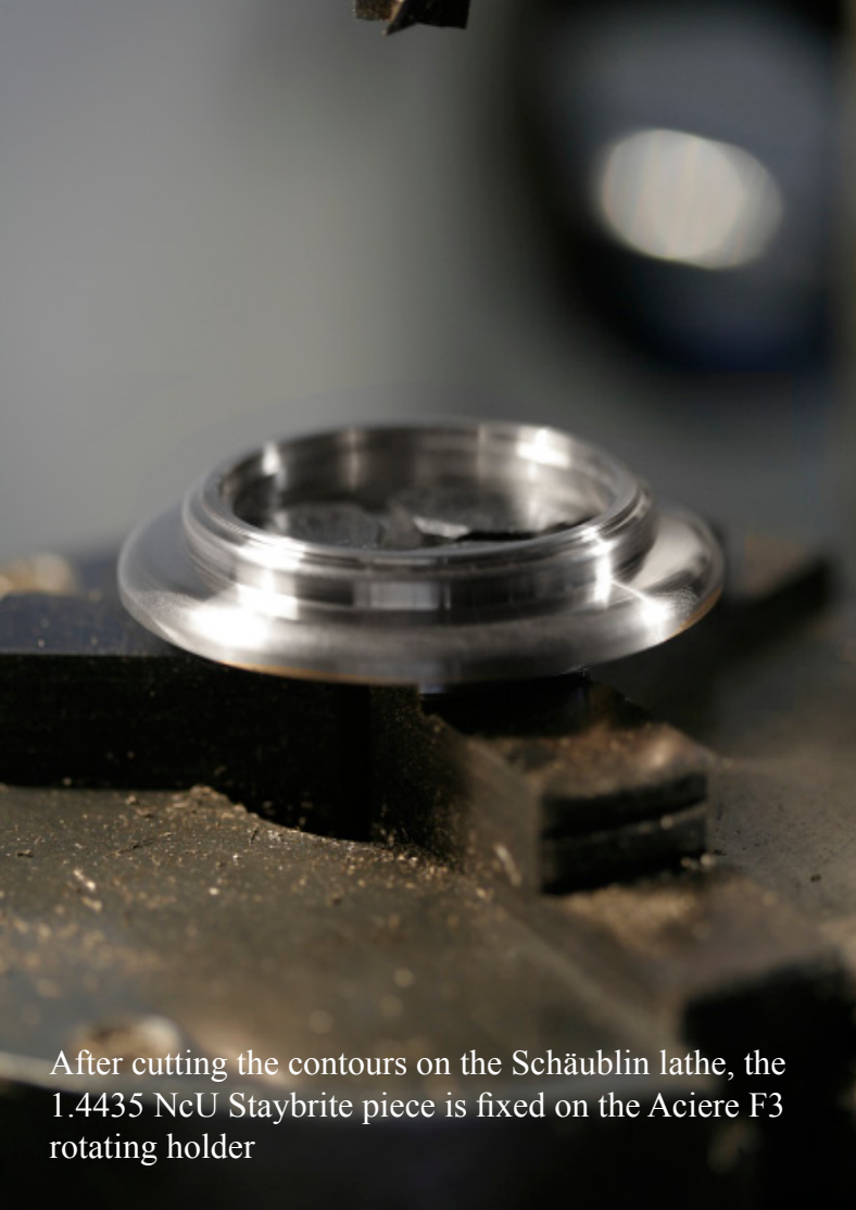
With a milling hjead of the diameter of the radius between case and corns, the left and right side of the case is milled out
