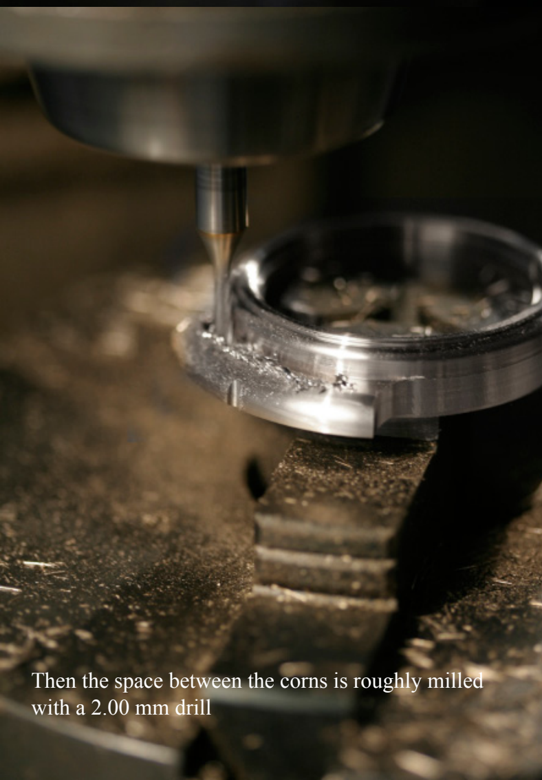
After cutting the contours on the Schäublin lathe, the 1.4435 NcU Staybrite piece is fixed on the Aciere F3 rotating holder
