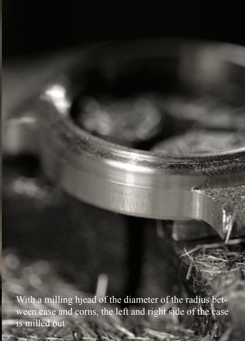
After cutting the contours on the Schäublin lathe, the 1.4435 NcU Staybrite piece is fixed on the Aciere F3 rotating holder
