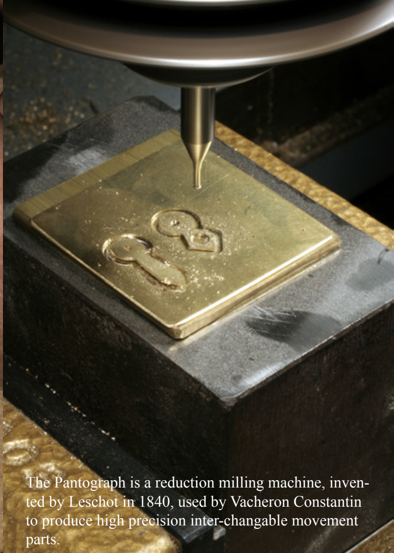
The Pantograph is a reduction milling machine, invented by Leschot in 1840, used by Vacheron Constantin to produce high precision inter-changable movement parts.
