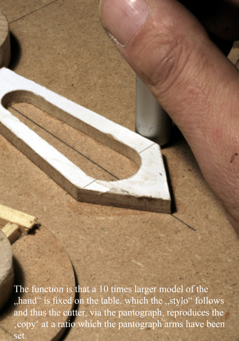
The Pantograph is a reduction milling machine, invented by Leschot in 1840, used by Vacheron Constantin to produce high precision inter-changable movement parts.
