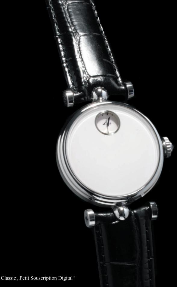
Circular two-body case, stainless steel Staybrite 1.4435 Cnu, mirror polished bezel, satin finished fluted sides, steel crown with cabochonOnix, sapphire crystal with golden round aperture for digital time display by "Souscription" hour disk, mechanical hand-winding movements, leather strap. Case caliber 39.00.00 mm
