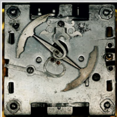
TOP VIEW OF MOVEMENT WITH FOLIOT
