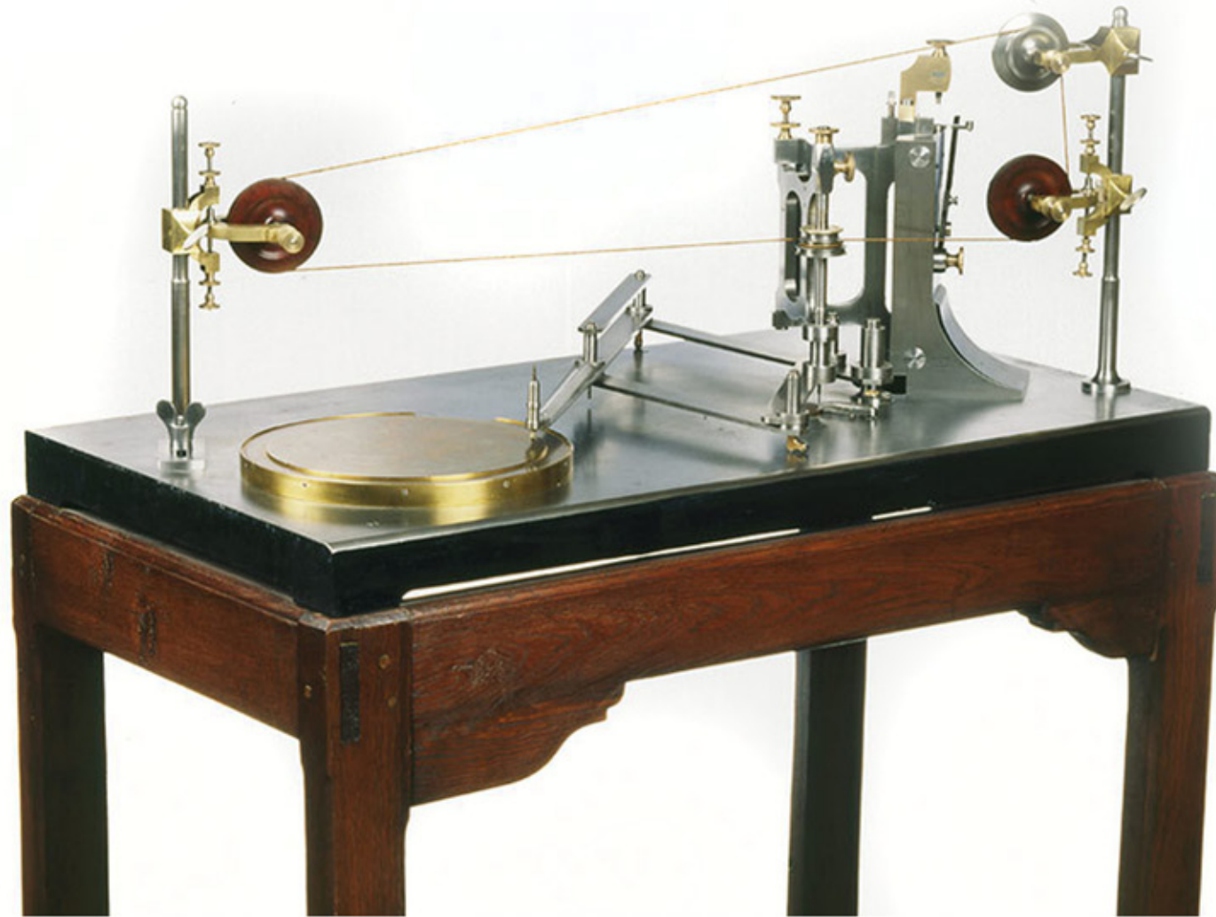
In 1841, Georges-Auguste Leschot began working with a pantograph at Vacheron Constantin. It used a matrix or pattern to mill identical and interchangeable watch plates and bridges.
