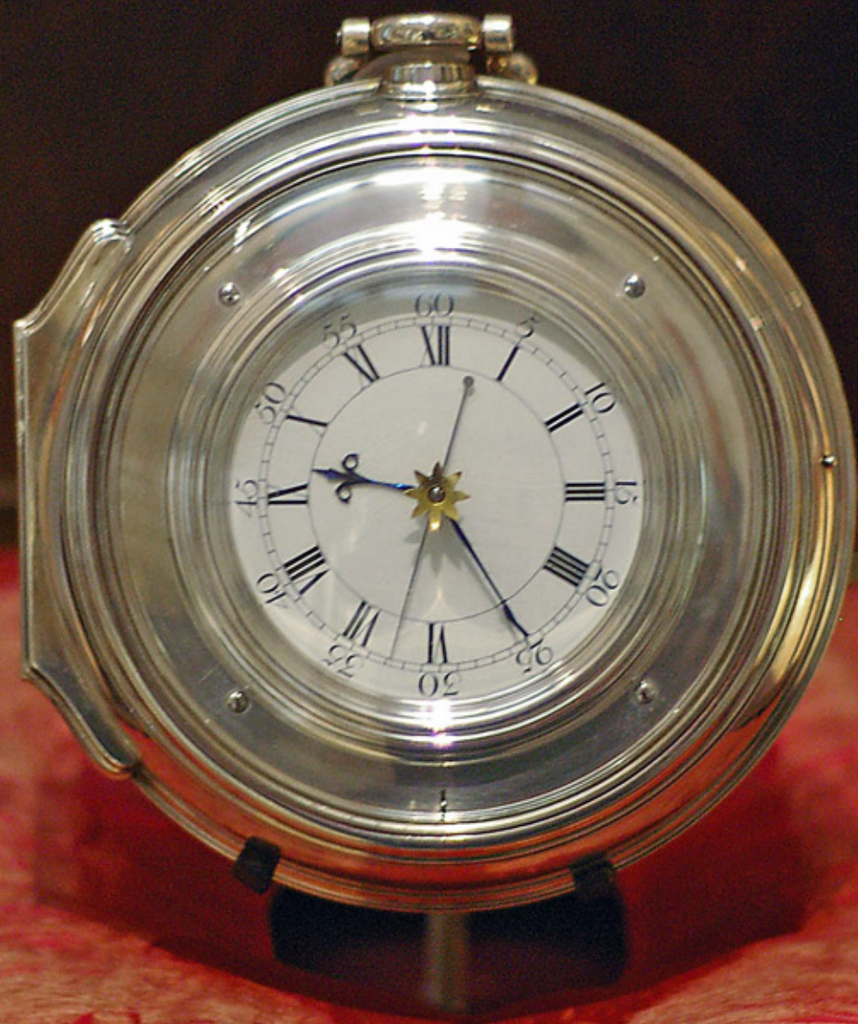
„Ship Watch“ H4 - Lost 5.1 seconds during a 14 month voyage from London to Jamaica Diameter 13.50 cm
