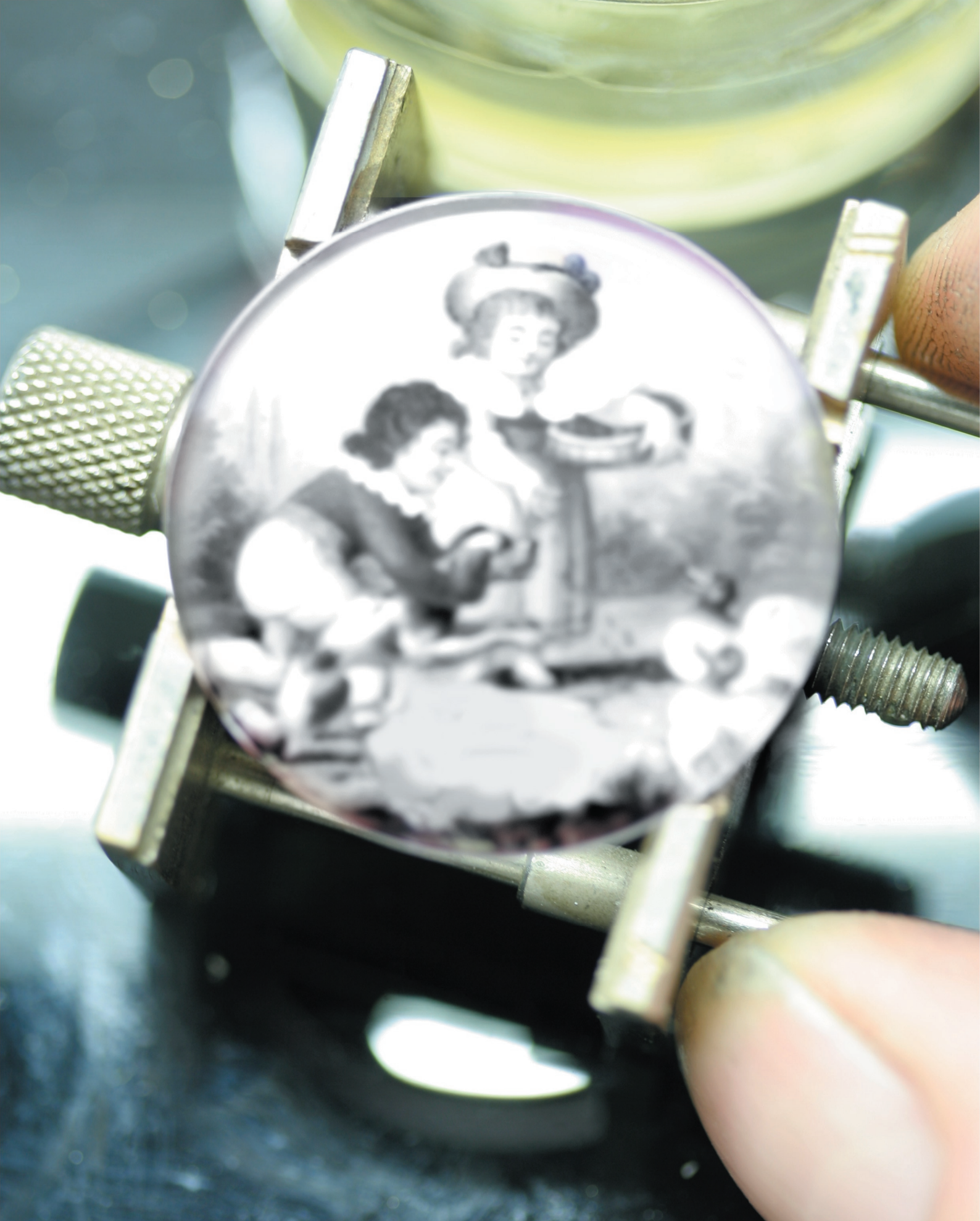
The sapphire crystal shown from the front side after black pigments have set
