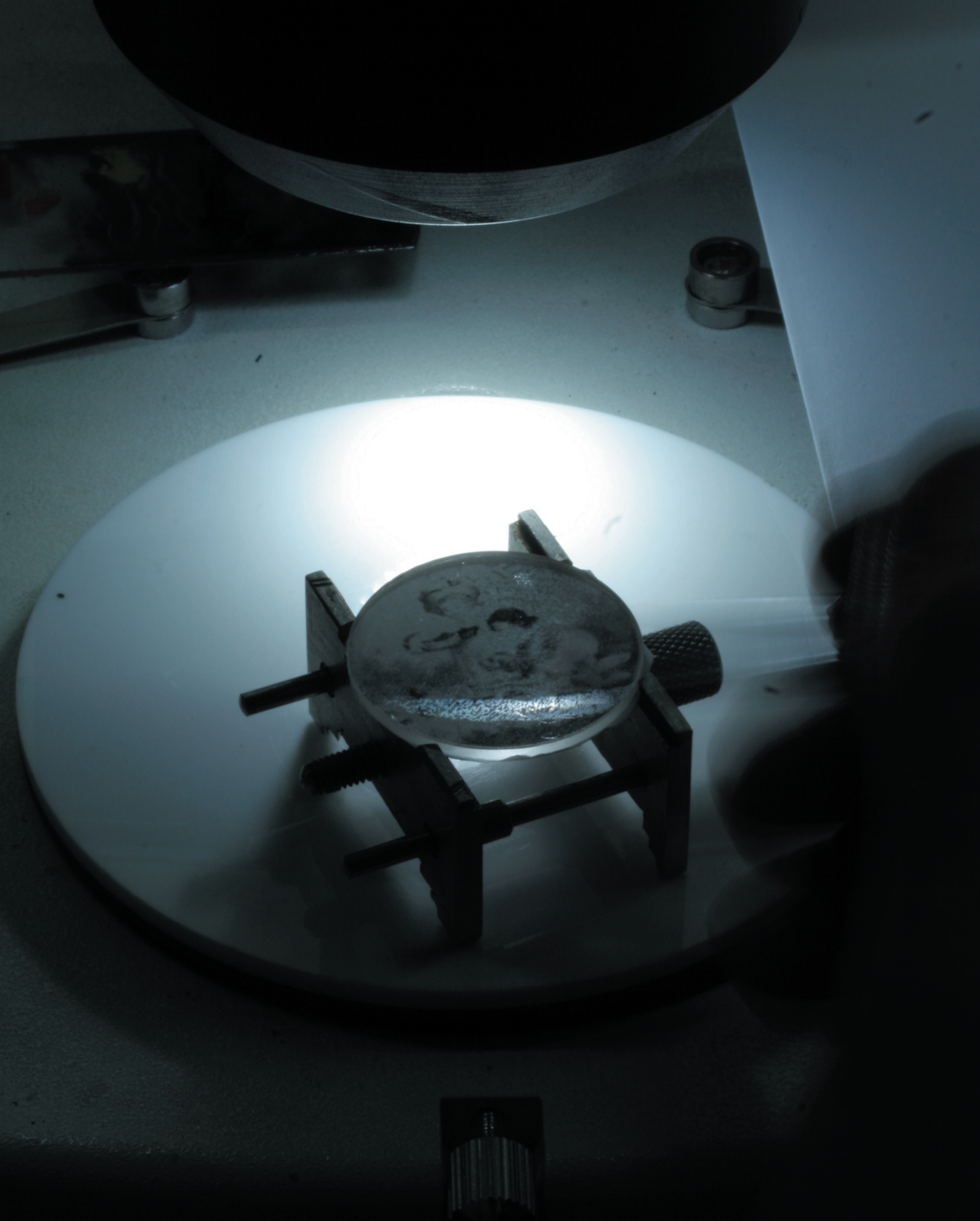
With a bush, a thin layer of Aqua Regia Oil is applied on the whole surface of the sapphire
